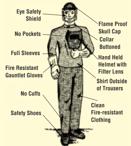
Personal Protective Equipments to be used during welding
