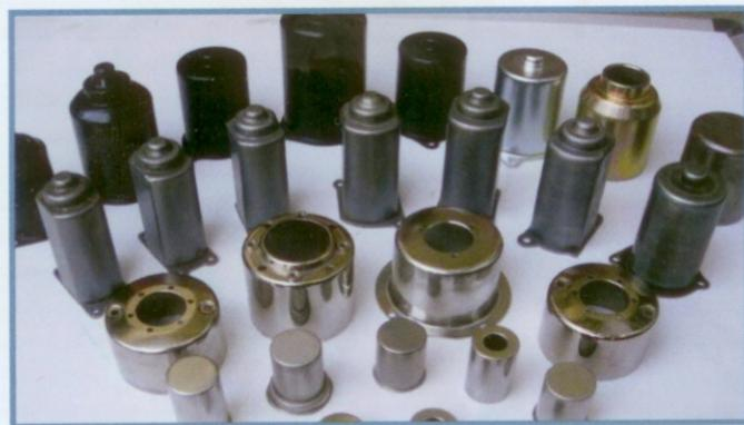
The company also manufactures yokes for wiper motors for all the motor vehicles, which are manufactured indigenously in the country. Although, at the commencement of its business, Kirti Pressings dealt in resistance welding machines, special purpose machines and deep drawn components, they soon
